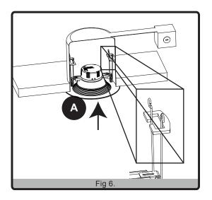
5. Carefully route wires into can fixture and hook both sets of spring clip arms into the arm hooks on the inside walls of the can, once secured inside the hooks, release spring clip arms and gently push the downlight (B) up into the can until flush against the ceiling surface.
