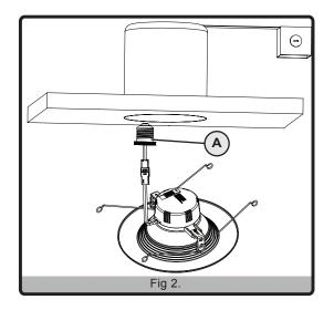
2. Make sure the power is turned off, Screw the adapter in luminaire (A) into existing socket in base.
