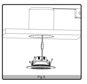
4. Squeeze the two sets of spring clip arms up towards each other and proceed to the next step to install the downlight into the can.
