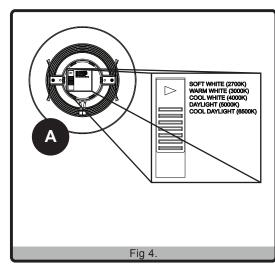
Before proceeding to the next step, set the desired color temperature (CCT), using the slide switch on the back of the housing. CCT can be changed from 2700K (soft white), 3000K (warm white), 4000K (cool white), 5000K (daylight), 6500K (cool daylight).
