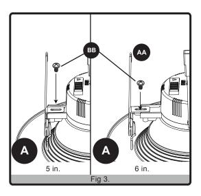
3. Adjust Spring clip arms (AA) to fit either 5" or 6" inch by screwing in screws (BB) at the demonstrated location on Fig.2. for desired can size.
